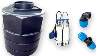
Primary Collection Tank Kit                    | 1x 1400 litre MDPE primary collection tank<br>1x 450mm access frame and cover<br>1x DN100 rubber pipe seal for pipe work connection<br>1x 240 volt stainless steel submersible pump c/w auto float control<br>1x set of 25mm (1") BSP pipe, valves, tank adaptor, non return valve, pressure relief valve and inline filter | <b>7052</b> |                      |
