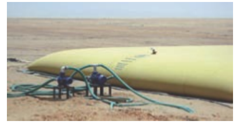
200 m 3 worksite water
