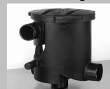
The above filter is a VF1 Combi filter which is suited to roof areas of upto 450m<sup>2</sup>. The rainwater flows from the roof the filter. The particles and debris are separated from the water. The clean water flows to the tank. The dirt is washed to waste or soakaway with a small amount of rainwater.
