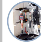
Flow meter, Hose and Nozzle
